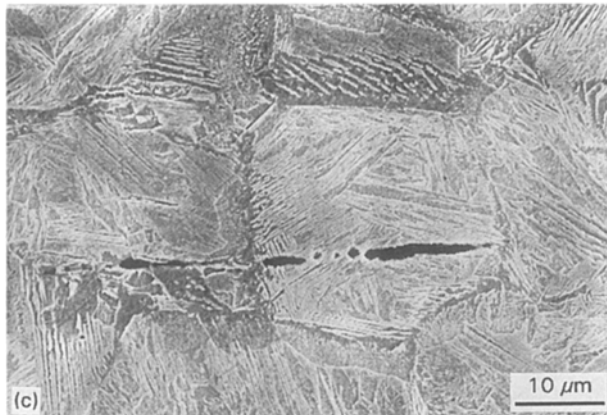
Figure 4 (a) The microstructure of HTWQ-LSM 1018 (b) higher magnification view of the same area, and (c) the microstructure of unmelted matrix material after water quenching.
