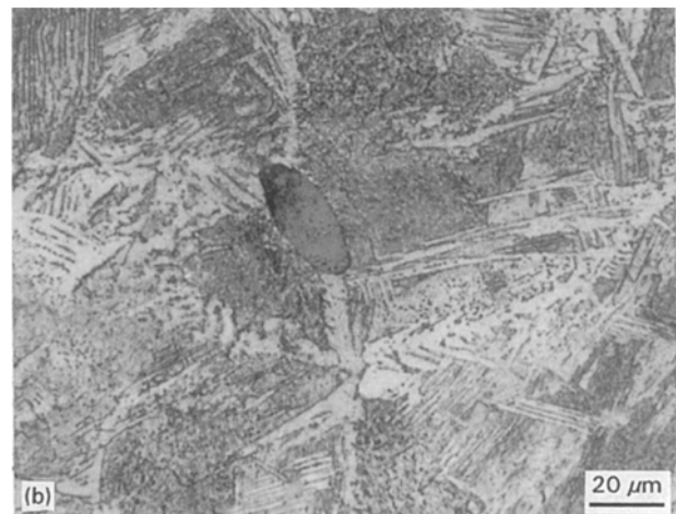
Figure 6 The microstructures of (a) melted and (b) matrix material after oil quenching.
